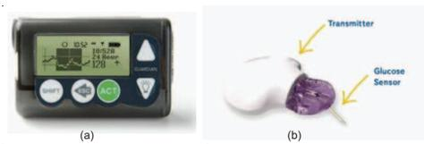
Fig. 4. Minimed sensor for continuous glucose measurement
